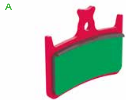
FIG A: A ridge left at the top of the pad shows that the wrong mount is used, and the caliper is sitting too high. Inversely a large unworn ridge on the outside of the disc shows the caliper is sitting too low. (More than 2mm)
