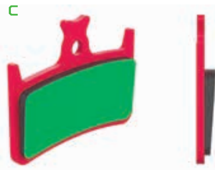
FIG C: A pad worn on a taper top to bottom is evidence of a warped disc.
