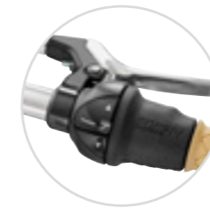
Rotating grip shifter with speed indication
