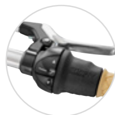
Rotating grip shifter with speed indication
